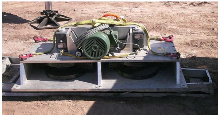
FIGURE 3.6. (From Star 2011) Mighty Mouse Eccentric Mass Shaker used for loading of test structure.
