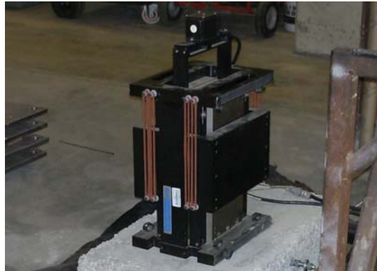
FIGURE 3.5. (From Star 2011) Picture of Atom Ant used for loading of SSI test structure.
